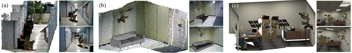
Fig. 15. Augmented reality (AR) applications. AR implementation and rendering results on the author-collected RGB-D dataset (a,b), and the ICL-NUIM dataset (c) with the animals, ISS, and sofa 3D objects. We exploit the 6-DoF camera pose tracking obtained by our proposed SLAM method as key information to render the 3D virtual objects in the real world. Note that any arbitrary 3D objects can be used.
